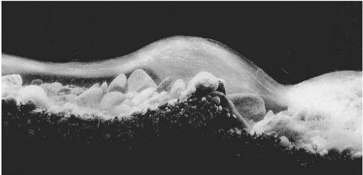
Figure 1 The flow over a step-pool structure. Photograph from Rosport [38].
