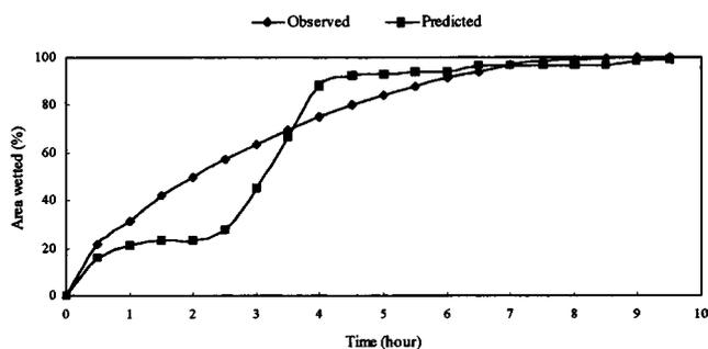
**Fig. 11.** Comparison of wetted area during advance for first basin
