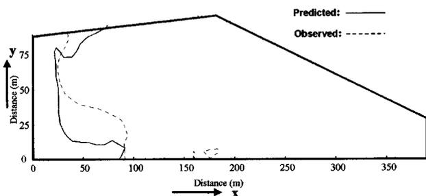
**Fig. 8.** Waterfront configuration after 30 min in first basin during first irrigation
