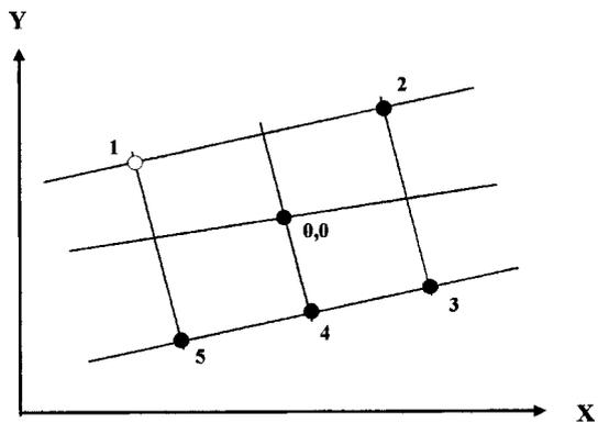
Fig. 4. Location of surrounding points for interior nodes
