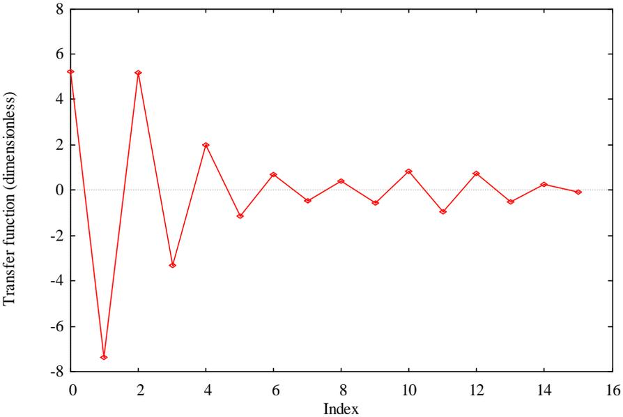
Figure 4: Inverse transfer function  $u_k$  for computing the gate stroking solution
