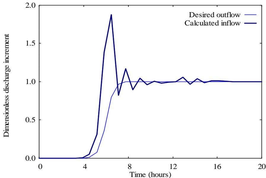
Figure 5: Outflow desired and the corresponding inflow required by the gate stroking solution where 90% of the flow increase occurs within an interval of 1.5 hours
