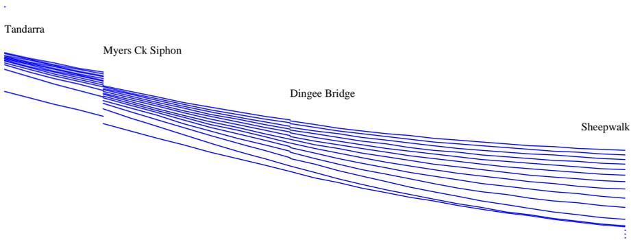
Figure 1: Water surface profiles in the first three pools of the Pyramid Hill No 1 Channel
