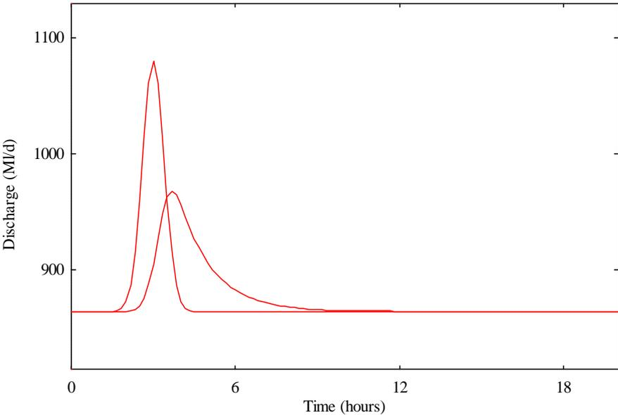
Figure 2: Specified inflow hydrograph and computed outflow hydrograph
