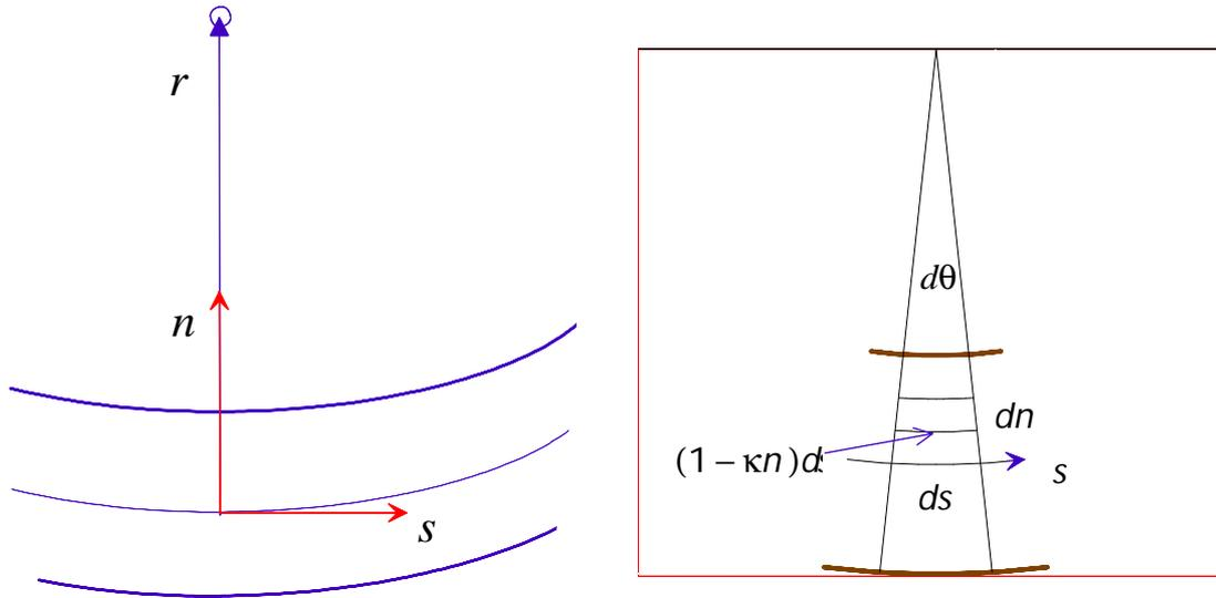
**Figure 1.** Orthogonal curvilinear coordinate system, physical dimensions, and control volume
