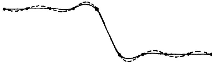
Figure 9. Interpolation near a discontinuity by: - - - finite Fourier series, – cubic splines.
