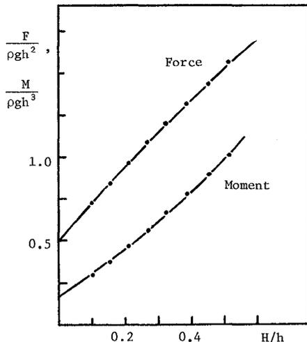
Figure 5. Maximum force and moment on the wall, plotted against incident wave height. The points ( $\bullet$ ) are numerical results from the present method to which curves have been fitted, as described in the text, shown by solid lines.
