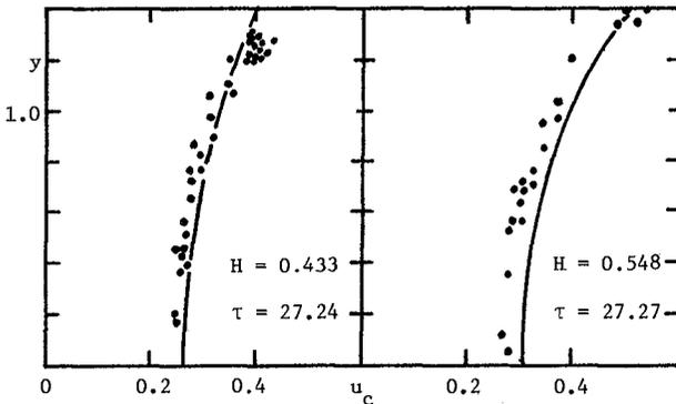
Figure 2. Horizontal fluid velocity under the wave crest,  $u_c$ , plotted against height  $y$  above the bottom: comparison between present method (—) and the experimental results of Le Méhauté et al (1968). Dimensionless wave heights and periods are shown.
