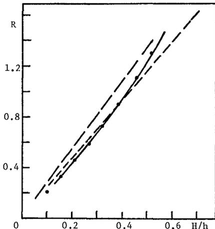
Figure 4. Maximum run-up at the wall  $R = (\eta_{max}/h) - 1$ , where  $h$  is undisturbed depth, plotted against incident wave height  $H/h$ . Points ( $\bullet$ ): numerical results from present method. (—): mean of experimental results reported by Chan & Street. (---): mean of experimental results from wave-wall reflection, and (- · -): wave-wave interaction, both from Maxworthy (1976).
