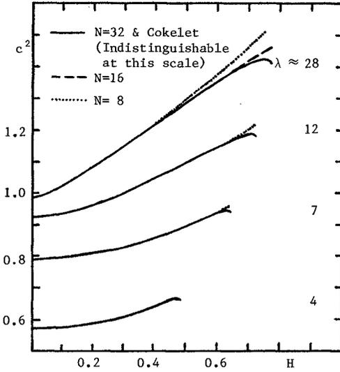
Figure 1. Comparison between the present method and the results of Cokelet (1977) for wave speed squared,  $c^2$ , as a function of wave height  $H$ . Each curve is drawn for a constant value of  $kQ/c$  taken from Cokelet's tables A2, A4, A6, A8, giving the almost constant values of wavelength shown.
