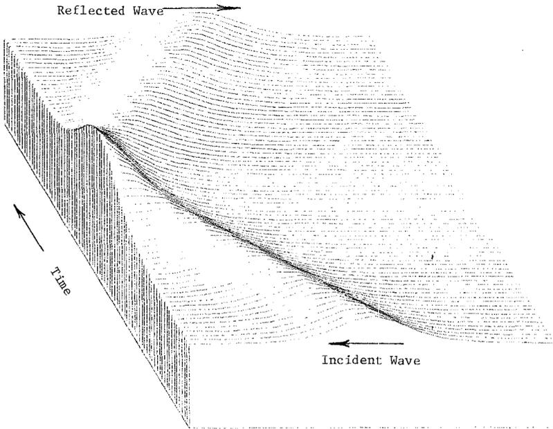
Figure 3. Surface elevation for a long wave of height 0.3 of the mean depth (approximating a solitary wave of height 0.325 above the trough), being reflected by a vertical wall at the left. Profiles are shown for successive times. Vertical exaggeration  $\approx 4:1$ .
