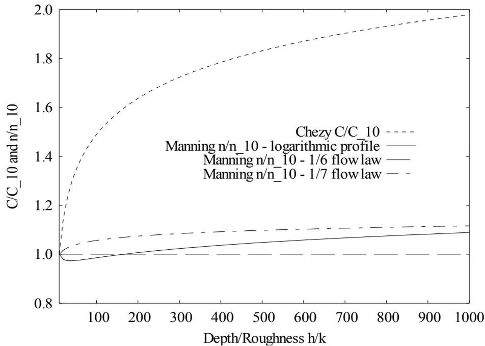
Figure 2. Variation of roughness coefficients with relative depth of flow
