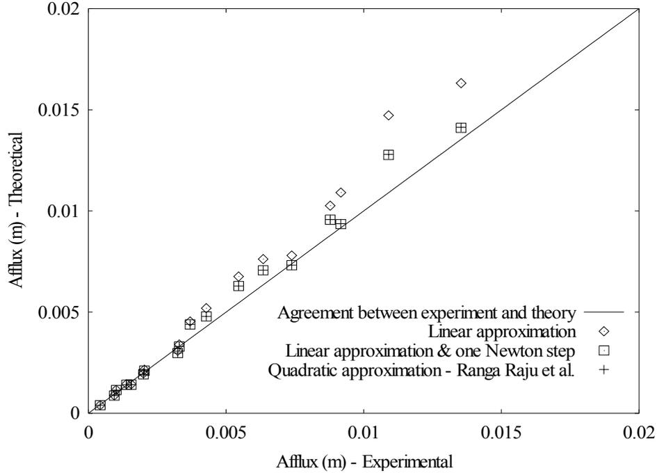
Figure 1. Change of surface elevation (afflux) across obstacle
