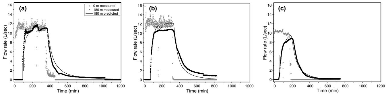
Fig. 4. Plot of measured and predicted flow rates in the farm drain for field investigations (a) 2:9-May-01, (b) 3:7-Jun-01, and (c) 4:31-Jul-01.
