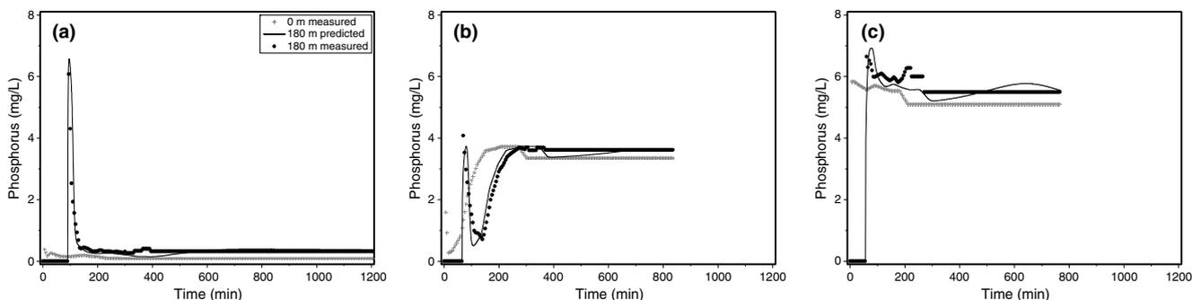
Fig. 6. Plot of measured and predicted phosphorus concentrations versus time in the ‘fenced’ drain on the Macalister Research Farm, using optimised coefficients for phosphorus uptake and release by bed sediments for experimental flows (a) 2:9-May-01, (b) 3:7-Jun-01, and (c) 4:31-Jul-01.
