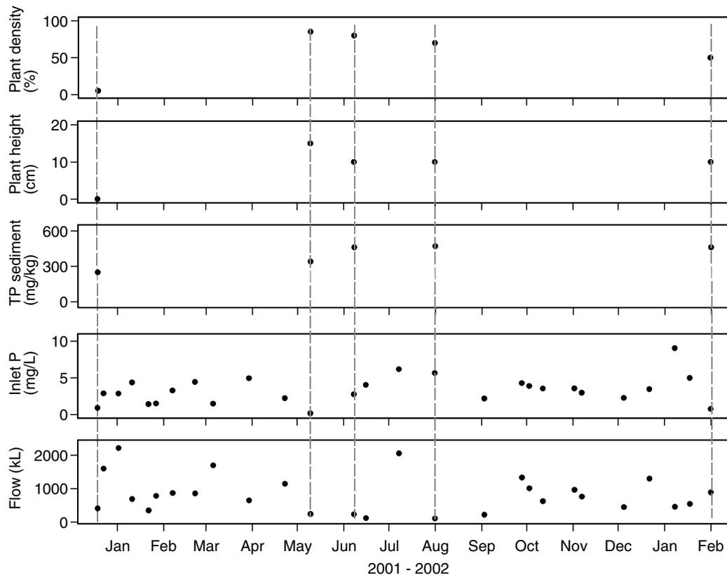
Fig. 2. Summary of sediment and plant characteristics as well as flow volumes and average inlet concentrations for field investigations and runoff events over the 14-month modelling period (vertical lines represent the timing of field investigations).
