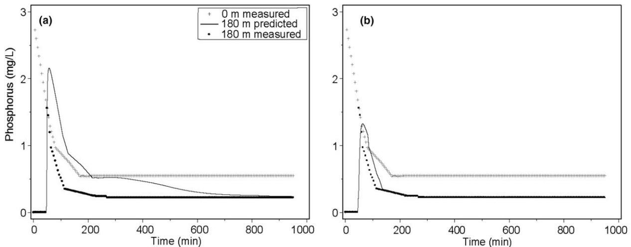
Fig. 5. Measured and predicted P concentrations versus time during the first field investigation (18-Dec-00), modelled using (a) laboratory based estimates of  $a_{\text{bed}}$ ,  $b_{\text{bed}}$  and EPC, and (b) optimised using  $a_{\text{bed}}$ ,  $b_{\text{bed}}$  and EPC.
