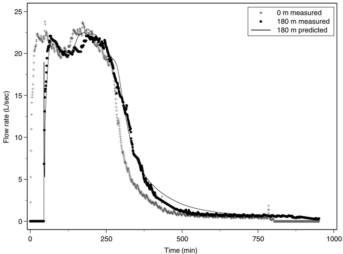
Fig. 3. Plot of measured and predicted flow rates in the farm drain for field investigation 1 (18-Dec-00) using a Manning's roughness of 0.011 and estimated infiltration coefficients.
