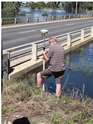
(c) GPS measuring water level and anxiously numerically differentiating with respect to time and extrapolating. The most important calculation!
