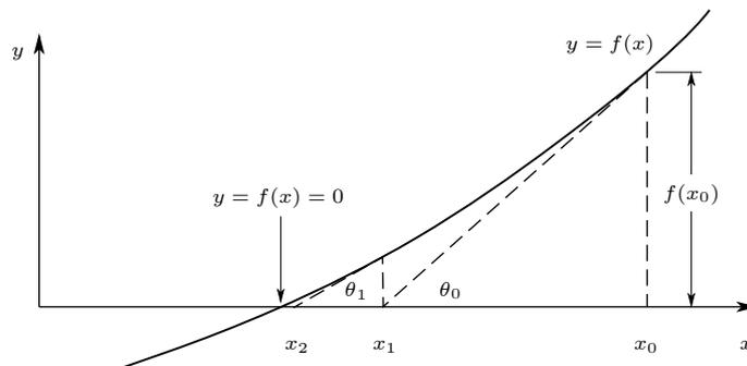
Figure 4-1. Newton's method
