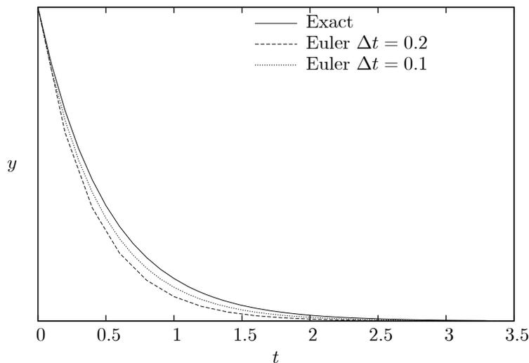
Figure 9-2. Comparison of results from Euler’s method
