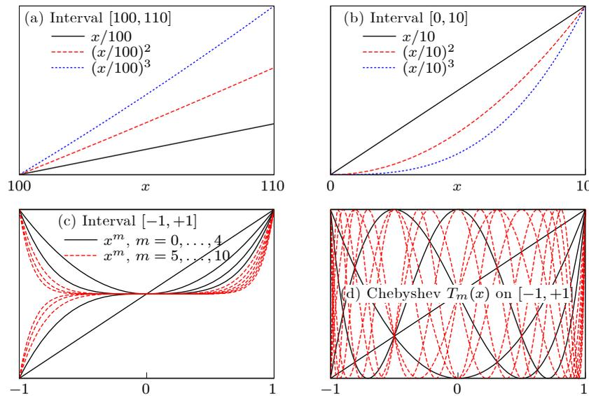
Figure 7-2. Comparison of the first three monomials on the intervals [100, 110] and [0, 10] and the first ten monomials and Chebyshev polynomials on [-1, +1]
