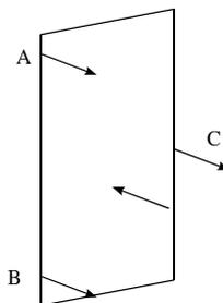
A vertical bulkhead in a ship has a door which has to be designed such that it will not be forced open if part of the ship fills with seawater of density  $1025 \text{ kg m}^{-3}$ . The door is 2 m high and 1 m wide, and the sea surface is assumed to be 1 m above the top of the door.
