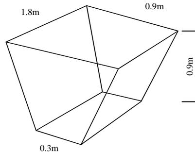
A mixing tank with trapezoidal ends is 1.8 m long, 0.9 m deep and 0.9 m wide at the top, tapering to 0.3 m wide at the base. If the tank is completely filled with water, calculate
