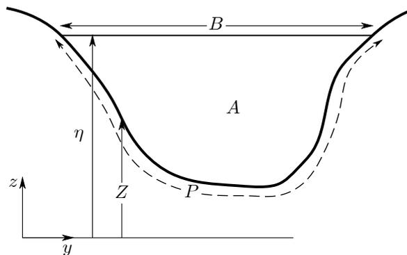
Figure 3-2. Cross-section of channel showing important dimensions
