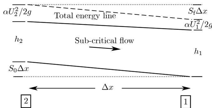
Figure 5-2. Elemental section of waterway
