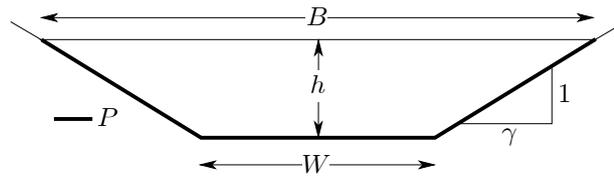
Figure 4-1. Trapezoidal section showing important dimensions
