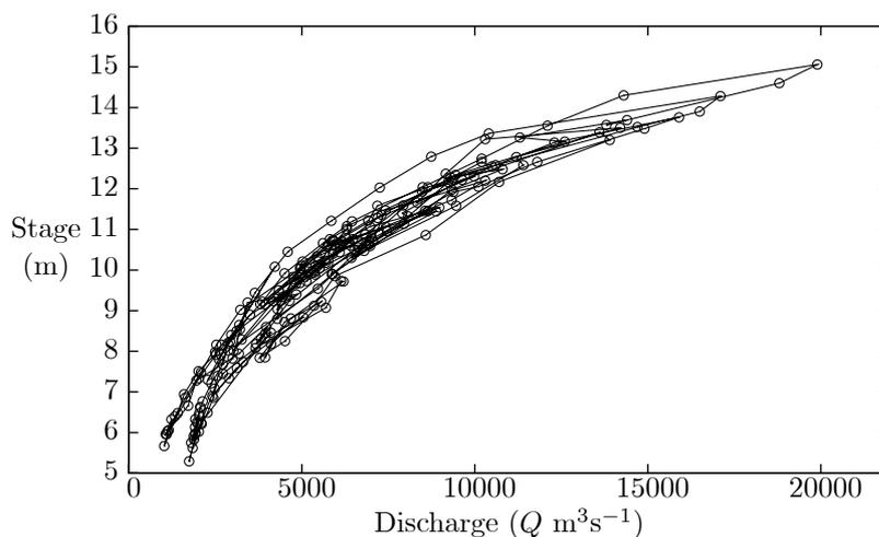
Figure 8-7. Flood trajectories for Station 41 on the Red River, showing raw data – corrected data was everywhere obscured
