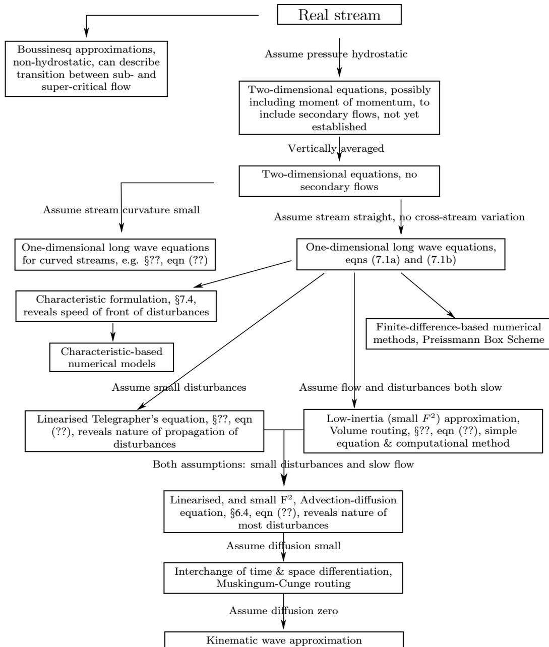
Figure 7-1. Hierarchy of one-dimensional open channel theories and approximations
