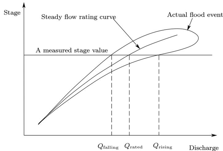
Figure 8-2. Stage-discharge diagram showing the steady-flow rating curve and an exaggerated looped trajectory of a particular flood event, which can be due to two effects: changing roughness and unsteady flow effects
