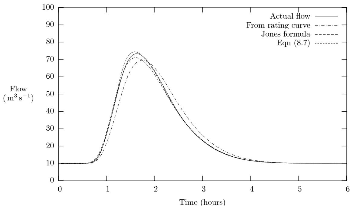
Figure 8-6. Simulated flood with hydrographs computed from stage record using three levels of approximation
