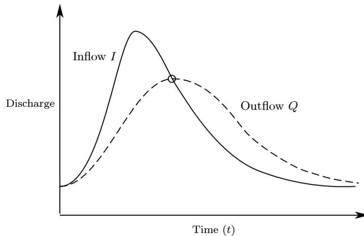
Figure 2-2. Typical inflow and outflow hydrographs for a reservoir
