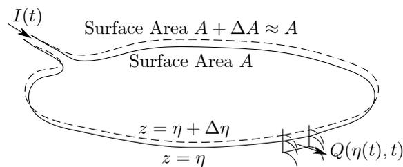
Figure 2-1. Reservoir or tank, showing surface level varying with inflow, determining the rate of outflow
