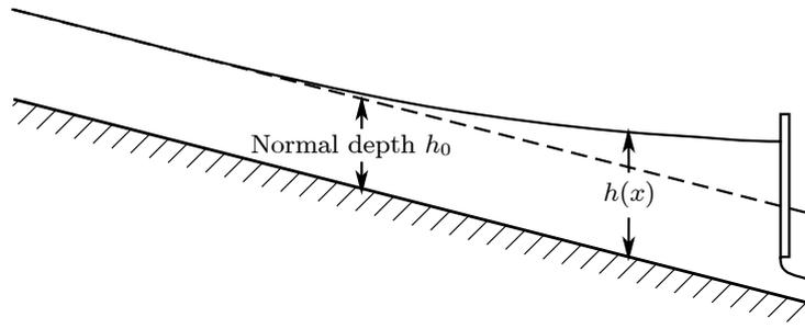
Figure 5-1. Subcritical flow retarded by a gate, showing typical behaviour of the free surface and, if the channel is prismatic, decaying upstream to normal depth
