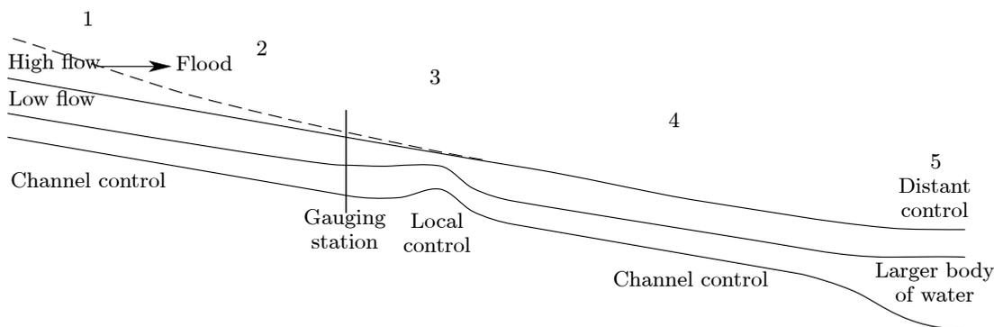
Figure 8-3. Section of river showing different controls at different water levels with implications for the stage discharge relationship at the gauging station shown
