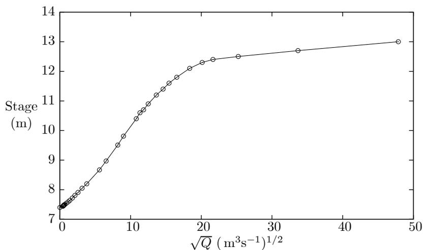
Figure 8-5. The same rating curve as in figure 8-4 but using  $(\sqrt{Q}, \eta)$  axes
