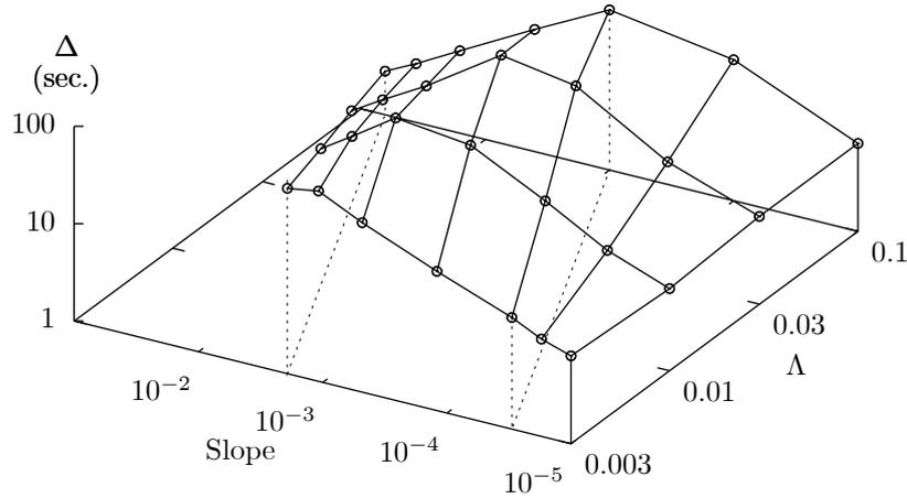
Figure 7-8. Stability limits determined by trial and error for a model river
