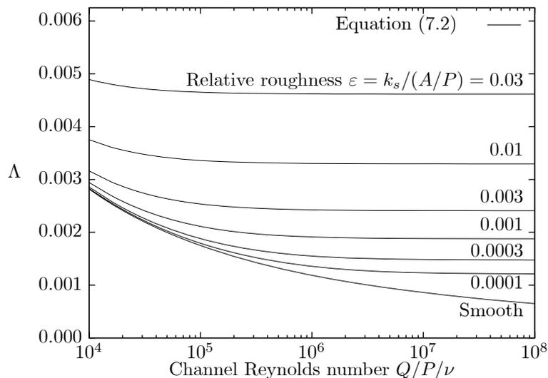
Figure 7-3. Dependence of  $\lambda$  on relative roughness and channel Reynolds number
