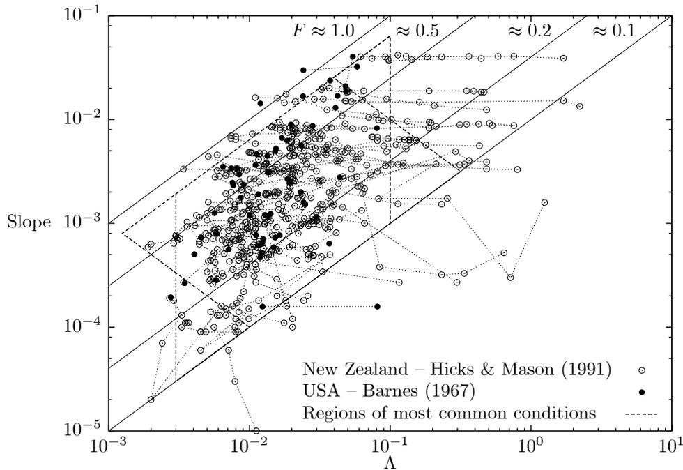
Figure 7-4. Resistance-Slope plot of rivers from New Zealand and the USA
