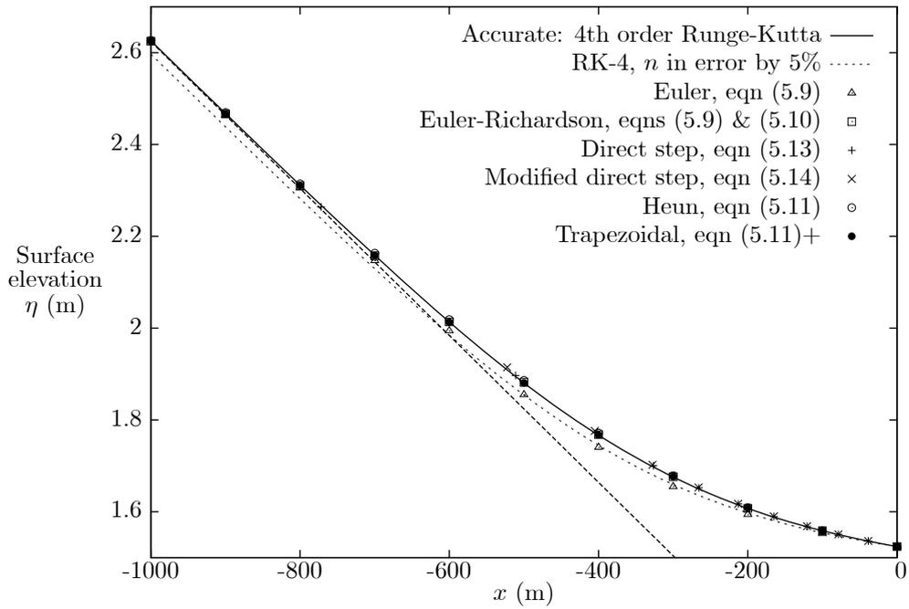
Figure 5-3. Backwater curve computed with various schemes; the dashed line is the surface for uniform flow.
