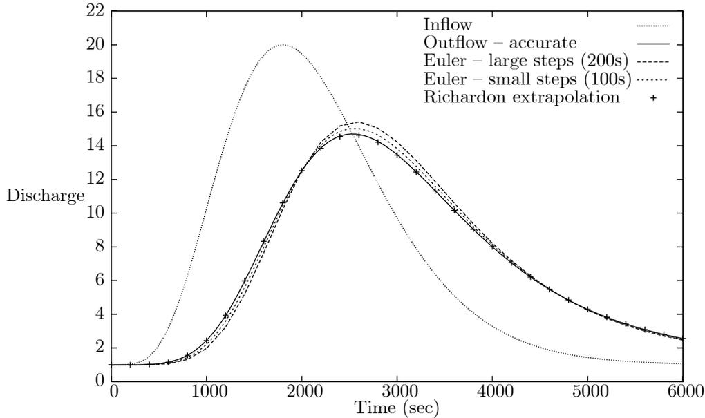
Figure 2-3. Computational results for the routing of a sudden storm through a small detention reservoir
