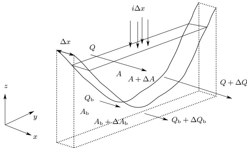
Figure 3-1. Elemental length of channel showing control volumes
