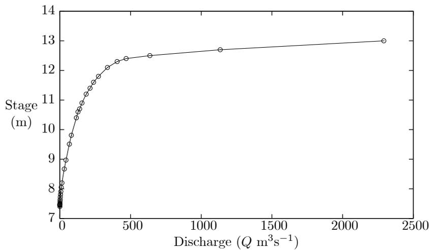
Figure 8-4. Rating curve using natural  $(Q, \eta)$  axes
