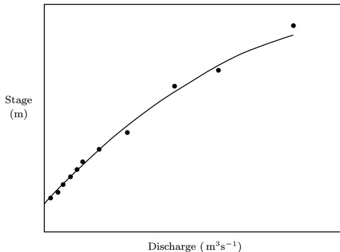
Figure 8-1. Rating curve (stage-discharge diagram) and data points to which it has been fitted
