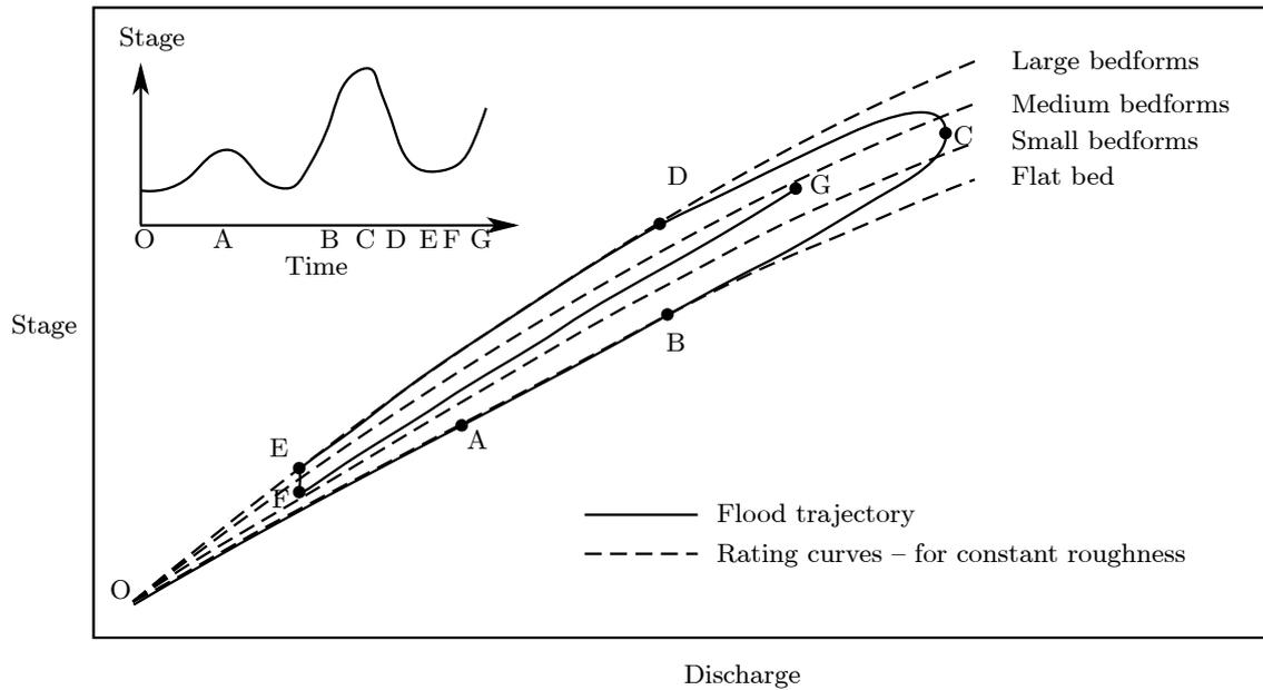
Figure 8-8. Rating curves for different bedforms and a looped flood trajectory
